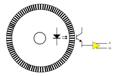
Figure 19. Representation of rotary shaft quadrature encoder
